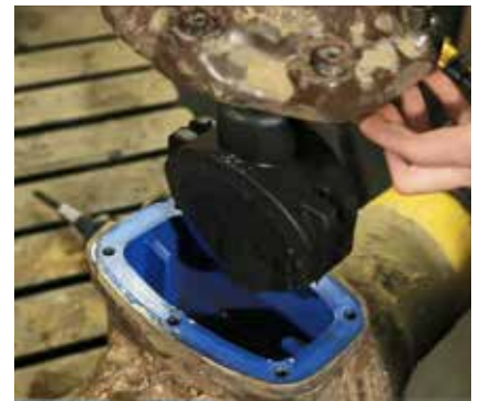
The photo above shows a fully functional PUR coated AVK valve produced in 1989 that has been excavated after 21 years of operation. The valve had to be opened by an angle grinder due to the robustness of the coating, and the valve was still in perfect condition.
